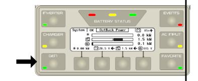
**To turn generator off:** Press the button under "Off."
